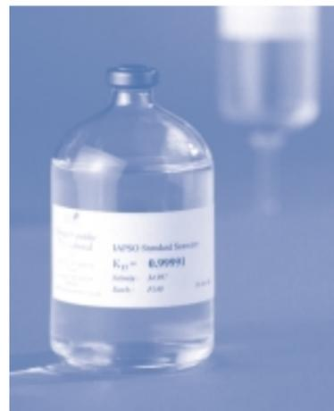
IAPSO Standard Seawater is available in sealed glass bottles, each containing ca.200ml of natural seawater. The bottle label carries information on its conductivity ratio (K15) and salinity according to the Practical Salinity Scale 1978 (PSS78).
